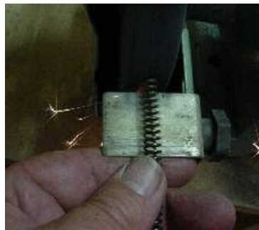
Figure 29: A trick I learned in replacing the mainspring is to use a kitchen fork. The center tongs of the fork fit nicely into the mainspring seat(5) and allow hammer strut(33) to pass through the center of the fork. With the hammer strut secured in the vise, I depress the fork and remove the paper clip. I gently back pressure off the fork as to control the spring. I then place the new spring on the hammer strut reapply pressure to the main spring seat with the fork and insert the paper clip back into the hole.
