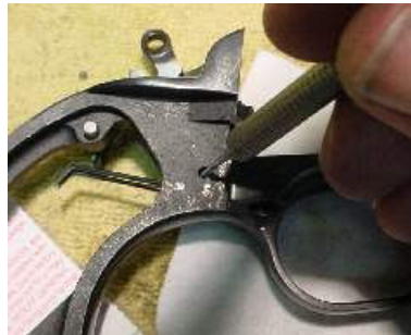
Figure 24: Then I use a punch to remove the trigger spring pivot pin (8). I then pull the trigger spring out the back of the grip frame.
