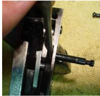
Figure 39: Using the punch as a guide I move the trigger pivot pin past each part until it clicks into place--the gate detent spring with the notch in the trigger pivot pin. At this pint I check to see if the gate detent spring is in place tight against the base of the loading gate. If not, I use a punch to push it into place
