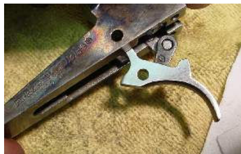
Figure 34: I attach the trigger to the transfer bar and rotate it into place in the cylinder frame.
