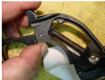
Figure 40: I place the main spring assembly into the grip frame making sure the "hump" is up.
