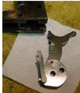
Figure 32: With the pawl attached to the hammer, I slide them past the transfer bar making sure the pawl slides along its channel and the transfer bar slides along its channel.
