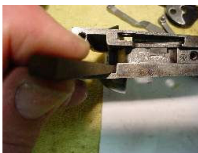
Figure 13: When stoning the cylinder frame I concentrate on 6 areas: the two channels where the pawl and the transfer bar slide, the areas where the trigger and hammer pivot, and the openings where the pawl and cylinder stop pass through the frame. Shown here I am stoning the pawl channel.
