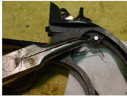
Figure 26: I reload the spring legs on the trigger spring retaining pin.
