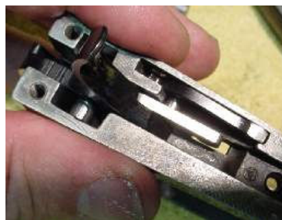
Figure 36: I then lift the gate detent spring slightly to allow the protrusion from the gate latch (5) to enter the center of the spring, then I slip the gate latch down beside the trigger.
