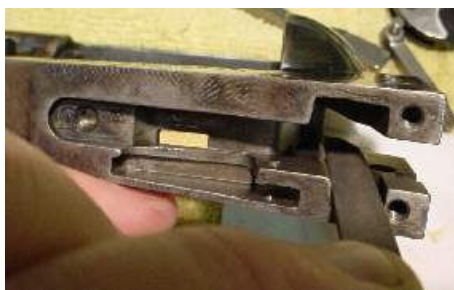
Figures 16-22: I stone parts where they move against the frame. I don't try to get an exactly smooth surface rather I try to get the high spots smooth so the parts will smoothly slide along the frame.
