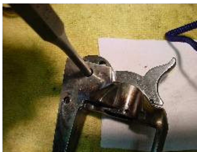
Figure 11: The hammer assembly comes out easily by tapping out the hammer pivot pin (29).
